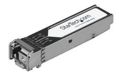
The 10056H-ST is an Extreme Networks 10056H compatible downstream fiber SFP transceiver which pairs with StarTech.com's 10057H-ST. They are designed, programmed and tested to work with 1000Base-BX-D compatible Extreme Networks switches and routers. The SFP transceiver module supports a maximum distance of up to 10 km (6.2 mi) and delivers dependable 1 GbE connectivity over fiber cabling.
